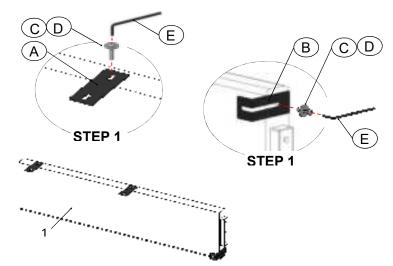
**STEP 2:** Attach brackets (A & B) facing right side to wing, to the end of the slot, using wrench(E), screw (C), and flat washers (D).
