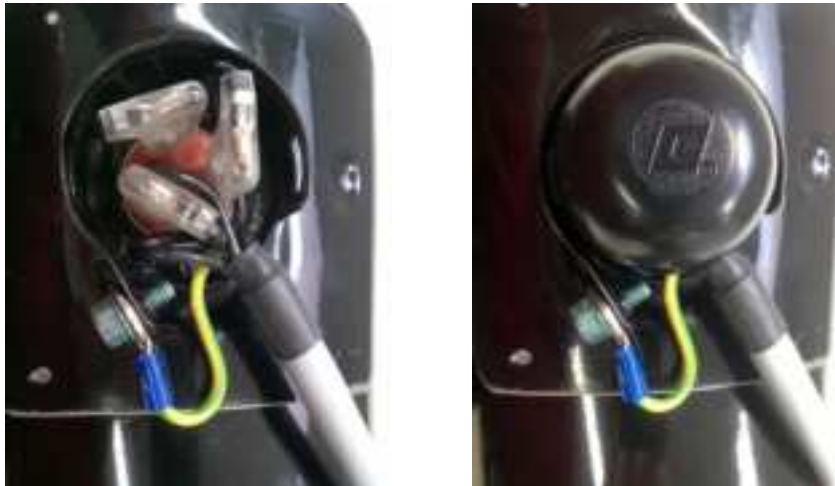
Figure 17: Terminal box and correct electrical installation
