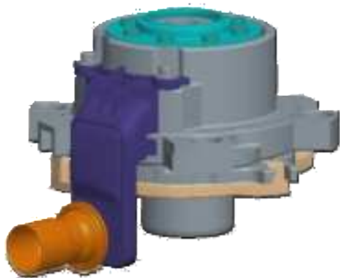
Figure 15: Suction funnel (purple part) in YHV*2P compressors
