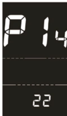
Current-limiting setting interface of the controller
