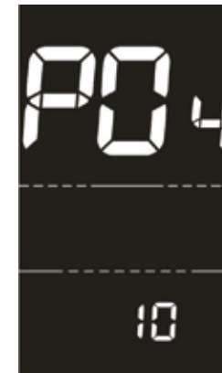
Automatic shutdown time setting interface
