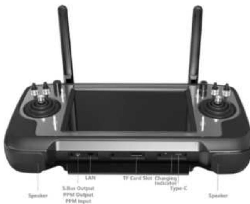
Overview – Ground Station Bottom
