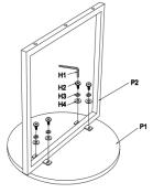
Step 2.Attach the table bottom(P3) to metal base(P2), using bolts (H2), lock washers (H3), flat washers (H4) tighten bolts with Allen wrench(H1) as illustration below.
