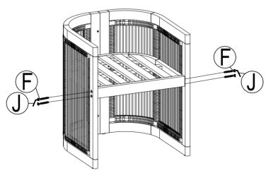
Use the Allen M4 (J) and screws (F) to connect the leg frame to the seat frame (A).
