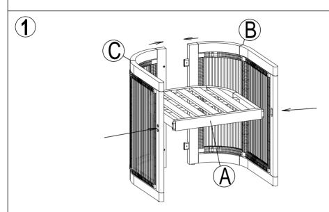
Take the leg frame 1 (B), leg frame 2 (C) and seat frame (A) and connect them together.
