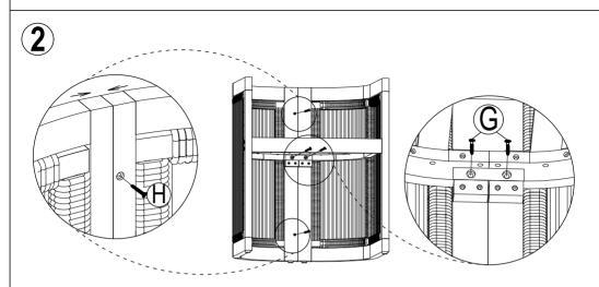
Use screw (H) to connect the two leg frames (C) and (B) together. Then use the Allen M4 (J) and screws (G) to connect the leg frame 1 (B) and the leg frame 2 (C).
