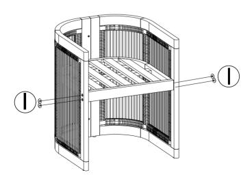
After tightening the screws, use the plastic lid (I). Cover the four screw heads.
