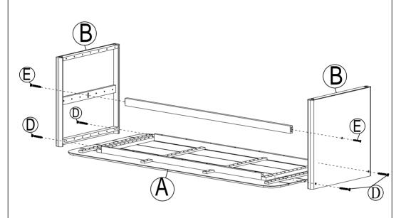
Use the Allen M4 (G) and Screws 7X90MM (D) to connect the Supporting Leg (B) with the Table Top (A)
