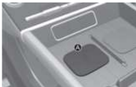
[A] Vehicle authentication pad (wireless charging pad)
