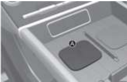
[A] Vehicle authentication pad (Wireless charging pad)
