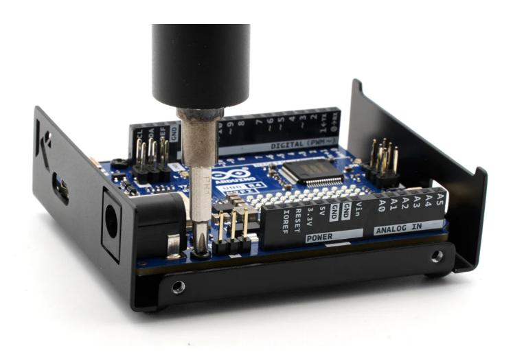
3. Close the lid and tighten the 4 countersunk screws.
