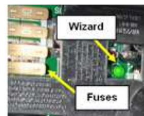
Wizard Button and Reverse Protection Fuses
