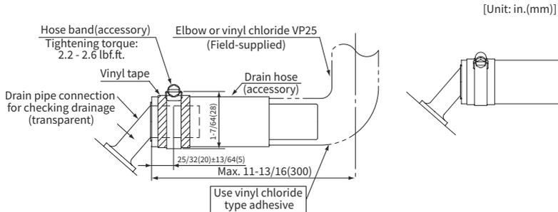
4. The condensate piping must be performed with a down-slope pitch of 1/25 to 1/100.
