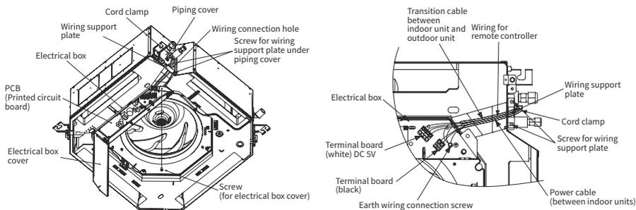
2. Remove the electrical box cover (1 screw).
