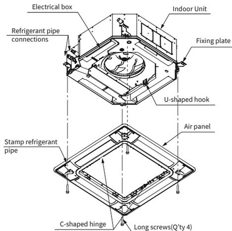
5. Tighten the long screws until touching the stopper to the fixing plate. Check to ensure that the distance between the fixing plate undersurface and the corner panel undersurface is 1-1/32in.(26mm).
