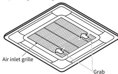
2. Hold the lower side of the air inlet grille keeping it inclined. Remove the hooks of air filter from the air inlet grille and remove the air filter.
