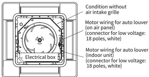
2. After connecting the wire connection of the air panel, attach the air inlet grille. Perform the attaching work in the reverse procedure of removing.
