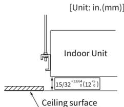
If not, adjust the distance by using the checking scale with maintaining the levelness of the indoor unit.
