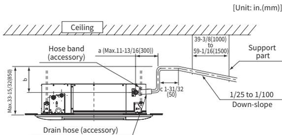
6. Do not apply excessive force to the condensate pipe connection. It could cause a damage.
