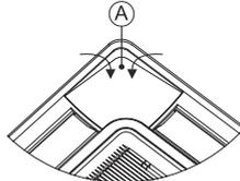
2. Pull down the U-shaped hook (at 2 positions) located at the indoor unit side.
