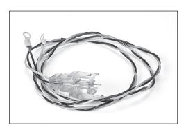
12.2 Plug the test probe into the cap of the pair being tested, with the black lead to the left and the red lead to the right.
