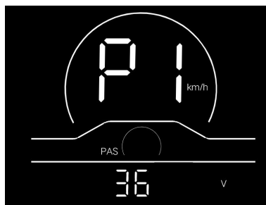
Fig. 7-1 Rated Voltage Setting Interface
