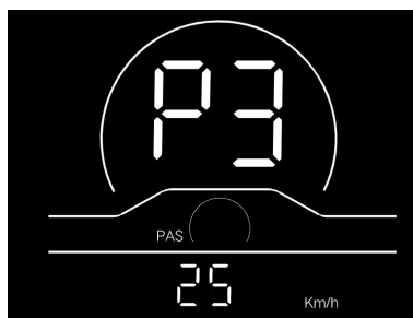
Fig. 7-3 Speed Limit Setting Interface
