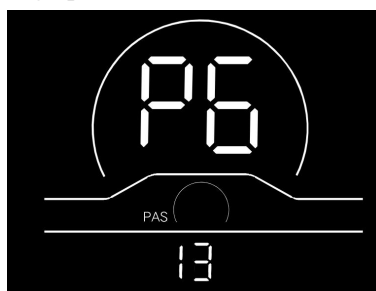
Fig. 7-6 Current Limit Setting Interface
