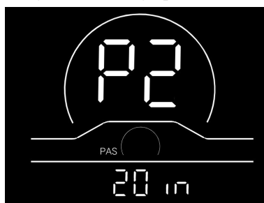
Fig. 7-2 Wheel Diameter Setting Interface
