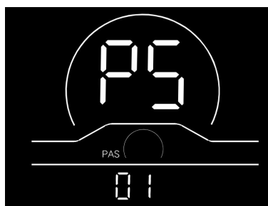
Fig. 7-5 Speed Sensor Setting Interface
