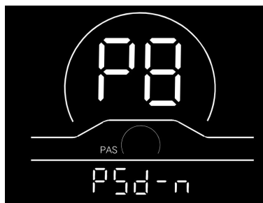
Fig. 7-8 Power-on Password Setting Interface
