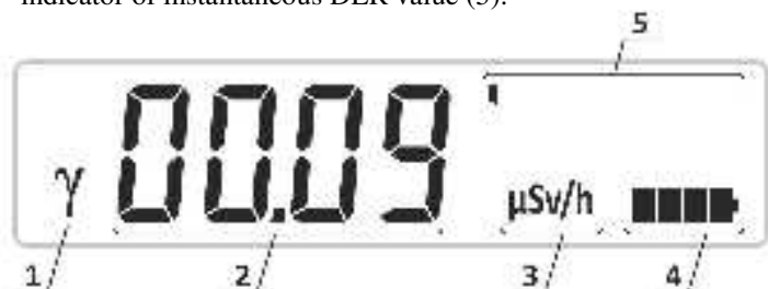
Figure 7 – LCD of the dosimeter (photon ionizing radiation DER measurement in search mode)
