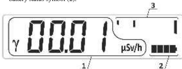
Figure 12 – LCD of the dosimeter (Measurement history viewing, measurement result display)
