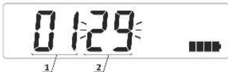
Figure 11 - LCD of the dosimeter (Viewing and setting measurement results averaging time for precise mode, and viewing statistical error of measurement result)
