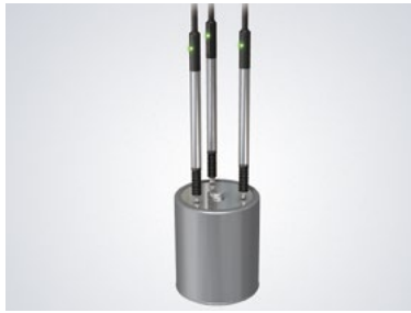
Battery flatness check
