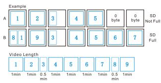
**Case A,** when the microSD card is not full, video "1", video "2", video "3", video "4", video "5" will be stored in the pre-allocated storage spaces in sequence. The remaining pre-allocated storage space will show 0-byte files.
