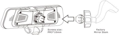
**Note:** If the diameter of the factory joint mount in your vehicle is 22mm, then you do not require the use of any Mount Adaptor Inserts.
