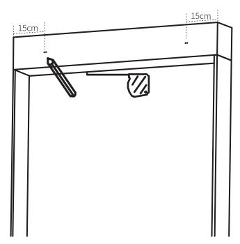
Step 2 Use the screws to anchor in the (pencil marked) bracket holes to firmly attach the mounting brackets to the surface.
