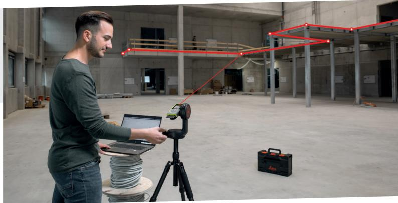
P2P Technology is a safe, accurate and efficient measurement method when it comes to distance measurements in inaccessible areas or complex measurement situations. It also enables a completely digital workflow, as the captured measurement results can be further processed in any CAD software.
