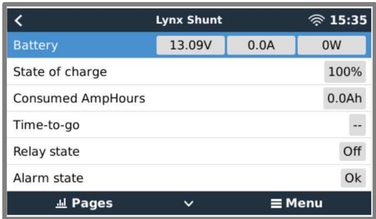
GX device displaying Lynx Shunt VE.Can operational data
