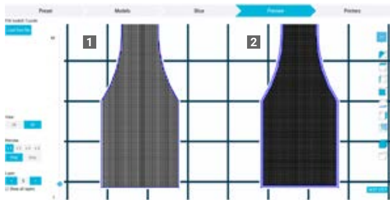
Fig. 2.15 The difference between a model printed with one perimeter line (1) and one printed with 2 perimeter lines with “Next perimeter offset” value set to 0.4 [mm](2).
