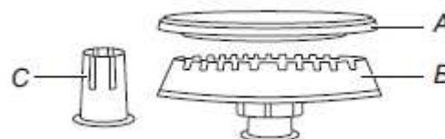
A. Burner cap B. Burner base C. Choke (for use with large burner, propane gas only)
