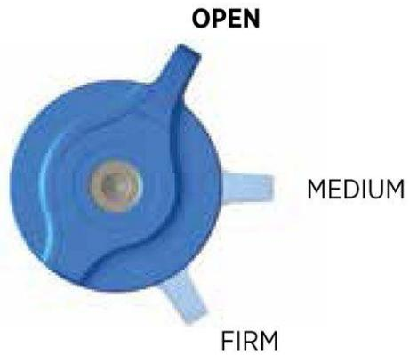
**\*OPEN Mode Adjust:** Open mode adjust is useful to control fork performance under rider weight shifts, G-outs, and slow inputs. OPEN mode adjust provides 22 additional fine tuning adjustments for the OPEN mode. Setting 22 will have a more plush feel and setting 1 will have a firmer feel.
