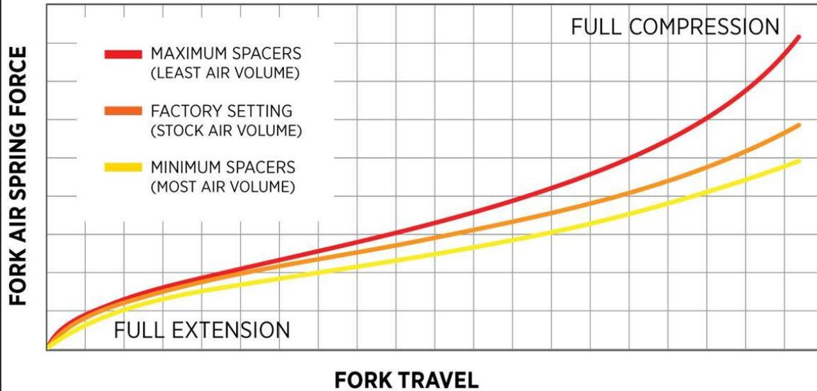
32 Step Cast FLOAT Volume Spacer Configuration
