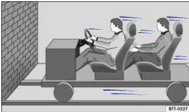
Fig. 68 A vehicle with passengers not wearing safety belts approaches a wall.
