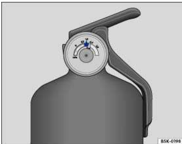
Fig. 193 On the fire extinguisher: Pressure gauge.
