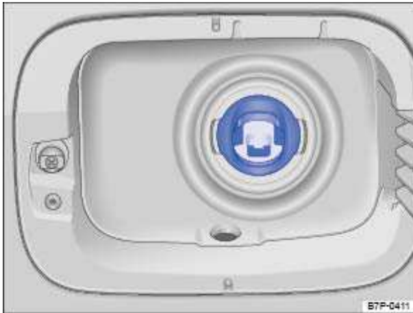
Fig. 163 With open fuel cap: Misfueling guard in the fuel filler neck.
