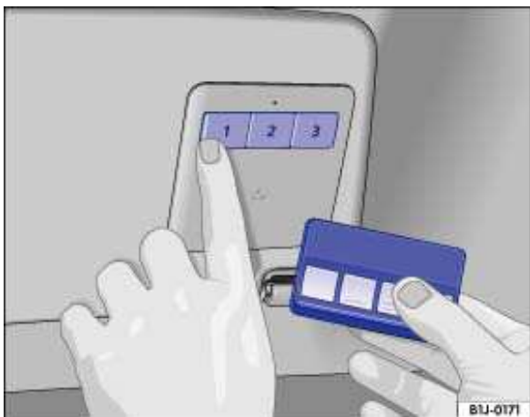
Fig. 51 To program: Simultaneously press the buttons for the HomeLink Universal Transmitter and the remote control.
