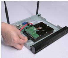
④ Connect the power wire
