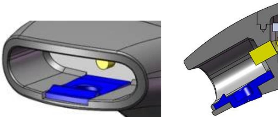
4. Fit the end of the strap into the end of the main body and push until the strap clicks in place.
