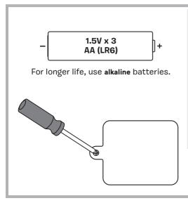
Loosen the screw in battery compartment door and remove the door. Remove the exhausted batteries and properly dispose. Insert three, new AA (LR6) **alkaline** batteries.
