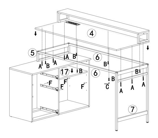
Fully tighten all screws using (C) at this time.
