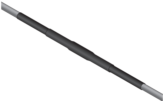
Figure 74: Completed joint with heat shrink seal
