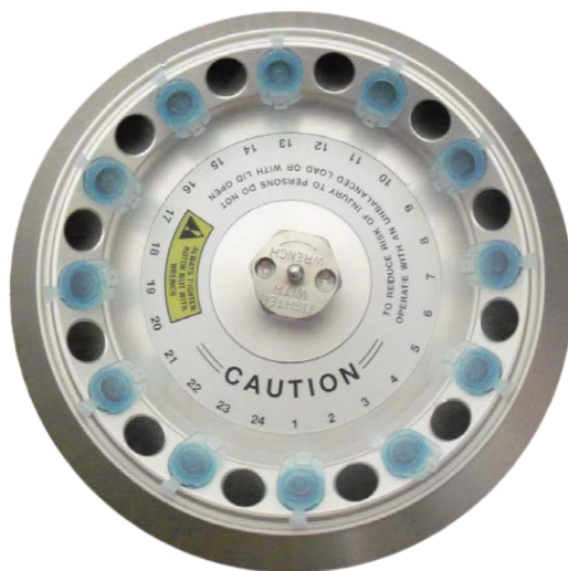
Figure 1. Loading the rotor to achieve balance.
