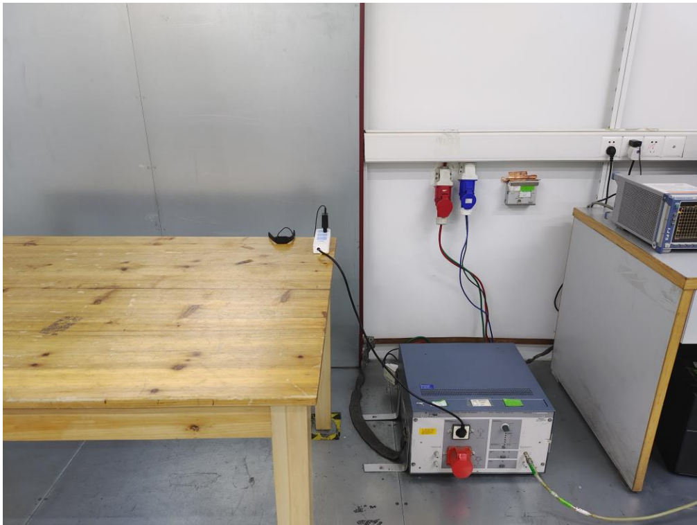
RADIATED EMISSION TEST SETUP (BELOW 1GHz)
