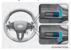
To resume Manual Speed Limit Assist after Manual Speed Limit Assist was paused, push the +, - switch or [] 5 button.
