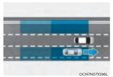
Blind-Spot Collision-Avoidance Assist helps detect and inform the driver that a vehicle is in the blind spot.
