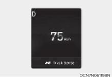
\* When N Track Sense Shift is operating, a message is displayed in the instrument cluster LCD screen as shown below.
