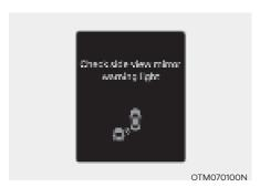
When the side view mirror warning light is not working properly, the 'Check side view mirror warning light' warning message will appear on the cluster for several seconds, and the master (A) warning light will illuminate on the cluster. If the master warning light illuminates, have the vehicle inspected by an authorized HYUNDAI dealer.
