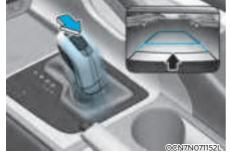
Rear View Monitor shows the area behind the vehicle to assist you when parking or backing up.
