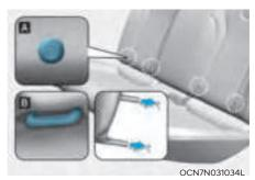
[A]: Lower Anchor Position Indicator[B]: Lower Anchor
