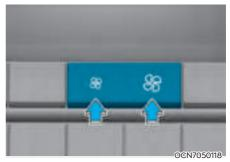
The fan speed can be set to the desired speed by using the fan speed control toggle switch.
