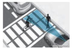
If there is a pedestrian(s) or bicycle(s) in between your vehicle and the vehicle in front, Leading Vehicle Departure Alert may not operate properly.
