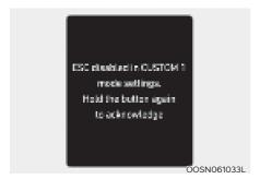
When N1 or N2 button is set to CUSTOM mode, you cannot turn CUSTOM mode on by pressing either N1 or N2 button if ESC OFF setting is saved within CUSTOM mode. If N1 or N2 button is pressed, a message "ESC disabled in CUSTOM 1 (or 2) mode settings. Hold the button again to acknowledge" appears on the cluster LCD display. To turn on CUSTOM mode with ESC OFF setting, press and hold N1 or N2 button.
