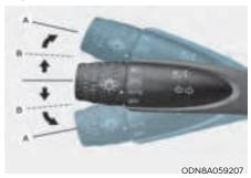
To signal a turn, push down on the lever for a left turn or up for a right turn in position (A). To signal a lane change, move the turn signal lever slightly and hold it in position (B). The lever will return to the OFF position when released or when the turn is completed.
