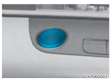
Whenever the front door is opened, the Engine Start/Stop button will illuminate and will go off 30 seconds after the door is closed. (if equipped)
