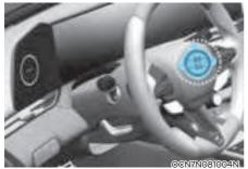
Detach the speed restriction label (0) from the sealant bottle (1), and place it in a highly visible place inside the vehicle such as on the steering wheel to remind the driver not to drive too fast.
