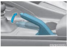
Always set the parking brake before leaving the vehicle, to apply: Firmly depress the brake pedal. Pull up the parking brake lever as far as possible.
