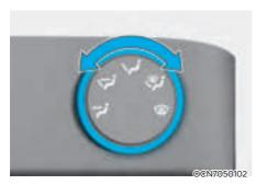
The mode selection knob controls the direction of the air flow through the ventilation system.
