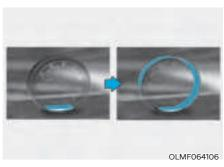
Immediately drive approximately 4~6 miles (7~10 km or, about 10min) to evenly distribute the sealant in the tire.
