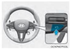
Push the II Switch to temporarily pause the set speed limit. The set speed limit will turn off but the Manual Speed Limit Assist enabled (© LIMIT) indicator will stay on.
