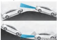
Blind-Spot Collision-Avoidance Assist may not operate properly when driving on a sloped road. The function may not detect the vehicle in the next lane or may incorrectly detect the ground or structure.
