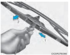
Lift up the wiper blade clip. Then pull down the blade assembly and remove it.
