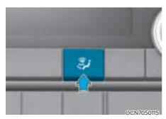
The mode selection toggle switch controls the direction of the air flow through the ventilation system.
