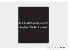
When the rear bumper around the rear corner radar or sensor is covered with foreign material, such as snow or rain, or installing a trailer or carrier, it can reduce the detecting performance and temporarily limit or disable Safe Exit Warning.
