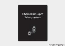
When Blind-Spot Collision-Avoidance Assist is not working properly, the 'Check Blind-Spot Safety system(s)' warning message will appear on the cluster for several seconds, and the master  $(\Lambda)$  warning light will illuminate on the cluster. If this occurs, have the vehicle inspected by an authorized HYUNDAI dealer.
