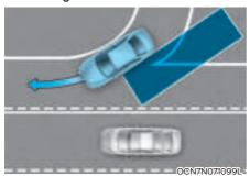
Blind-Spot Collision-Avoidance Assist may not operate properly when driving where the road merges or divides. The function may not detect the vehicle in the next lane. Always pay attention to road and driving conditions while driving.
