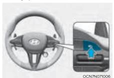
1. Press and hold Driving Assist button at the desired speed. The Manual Speed Limit Assist enabled (SILIMIT) indicator will illuminate on the cluster.
