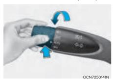
High Beam Assist will automatically adjust the headlight range (switches between high beam and low beam) depending on the brightness of detected vehicles and certain road conditions.
