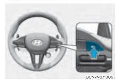
Press the Driving Assist button to turn Manual Speed Limit Assist off. The Manual Speed Limit Assist enabled (③) [IMIT] indicator will go off.
