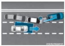
When changing lanes by detecting the lane ahead, if Blind-Spot Collision-Avoidance Assist judges that there is a collision risk with an approaching vehicle in the blind spot, it can help avoid a collision by applying the brake.
