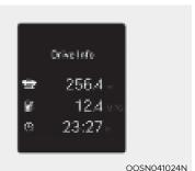
The trip computer mode displays information related to vehicle driving parameters including fuel economy, tripmeter information and vehicle speed.
