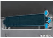
Remove the cabin air filter case while pressing the lock on the right side of the cover.
