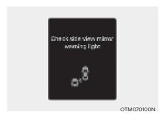
When the side view mirror warning light is not working properly, the 'Check side view mirror warning light' warning message will appear on the cluster for several seconds, and the master (A) warning light will illuminate on the cluster. If this occurs, have the vehicle inspected by an authorized HYUNDAI dealer.
