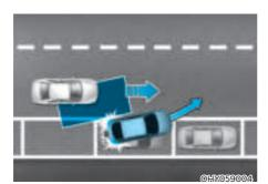
When you are driving forward out of a parking space, if Blind-Spot Collision-Avoidance Assist judges that there is a collision risk with an approaching vehicle in the blind spot, it can help avoid a collision by applying the brake.
