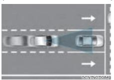
Forward Collision-Avoidance Assist is designed to help detect and monitor the vehicle ahead or detect a pedestrian in the roadway and warn the driver that a collision is imminent with a warning, audible emergency braking.
