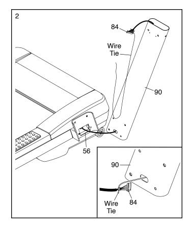
Hold the Right Upright (90) against the Frame (56). Be careful not to pinch the wires. Start a 3/8" x 4 1/4" Screw (43) with a 3/8" Star Washer (12) into the Right Upright and into the Frame; do not fully tighten the Screw yet.
