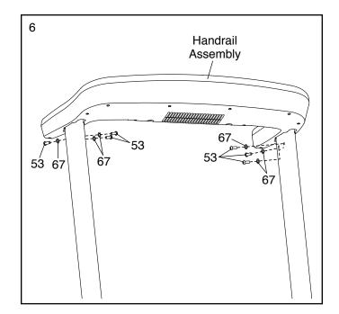
With the help of a second person, hold the console assembly near the handrail assembly. Be careful not to pull on the wires.
