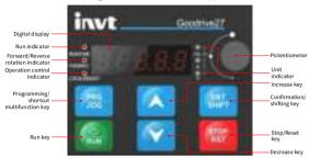
Figure 5-1 Standard LED keypad
