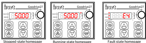
Figure 5-2 Status interface display
