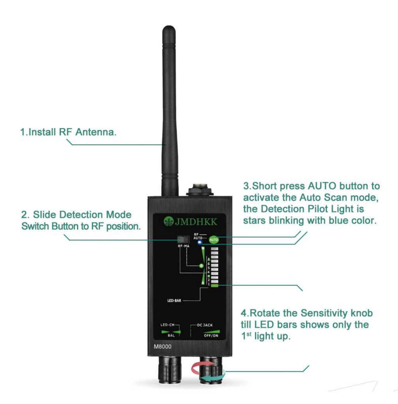
Note: Auto Scan can take several seconds or minutes depending on the RF signal strength in your surrounding and the distance between the detector and the transmission source. The stronger the RF signals are, or the shorter the distance is, the shorter time it will take for Auto Scan, it is the most convenient and effective way to find the transmitting bug devices in your surroundings.
