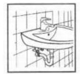
2. Temporarily place the half-pedestal against the basin and mark the mounting positions on the wall.
