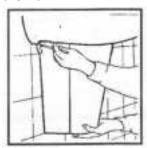
3. Fix the half-pedestal on the previously bored positions with the bolts.
