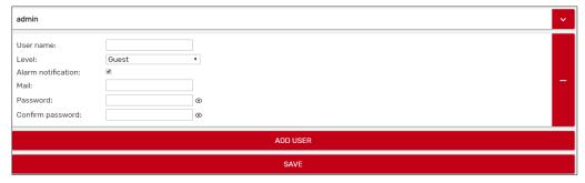
Select the *Alarm Notification* check box to send notification emails to the user when alarms occur in any device in the CANbus network enabled to send email (see *3.3 Network Configuration*).
