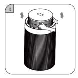
Take out the new filter with plastic film inside the body
