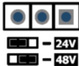
Fig.6. Setting voltage trigger for the brake circuit
