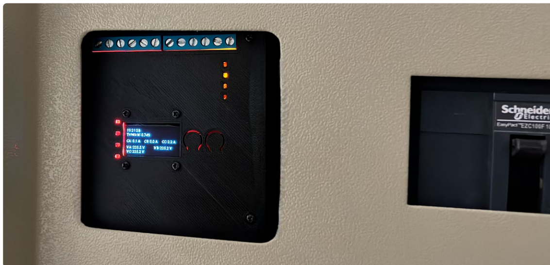
Figure 10: ESP32 Energy Meter installed in a circuit breaker panel, monitoring real-time power consumption.
