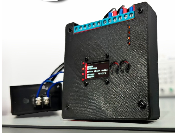
Figure 1: The assembled ESP32 Energy Meter with its OLED display and live status indicators.
