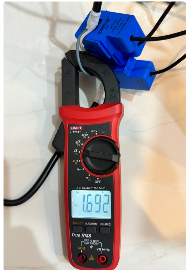
Figure 8: Clamp meter setup for calibration.
