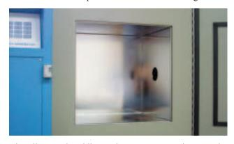
Virtually any humidity and temperature point may be generated, for any length of time, within the operational limits of the generator. The output of the device under test may then be compared with the generator's printed data for analysis.
