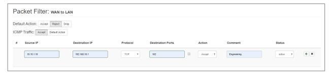
**Source IP** indicates the IP address of the active device in the company network (WAN).
