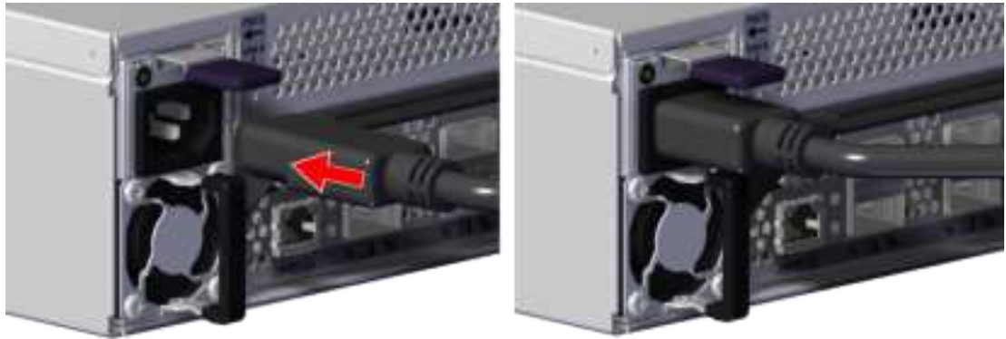
Figure 18: Connect Power Cable
