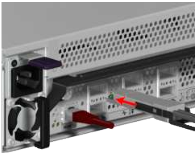
Figure 17: Connect QSFP28 Cable
