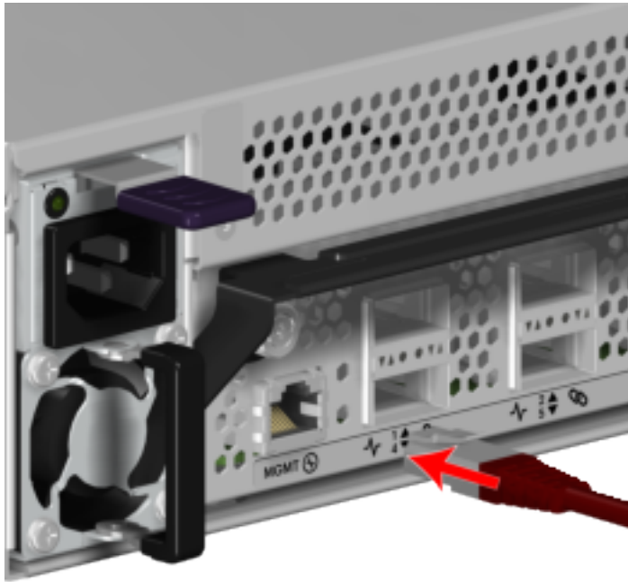
Figure 16: Connect Ethernet Cable
