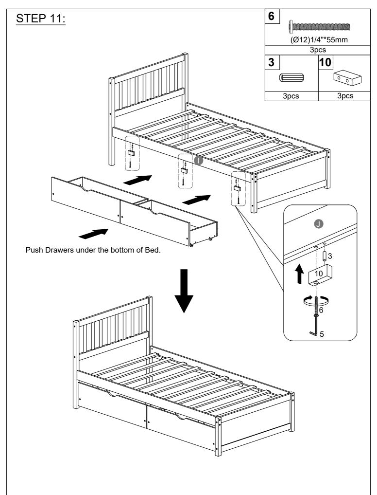
Make sure to tighten all the screws of the bed.
