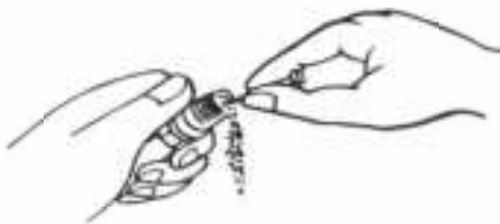
(2)clean carbon laydown
