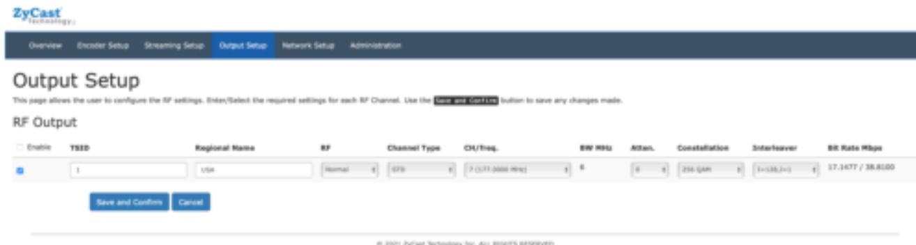
Use the Output Setup page to set the RF output type, RF Output CH/frequency, Attenuation, QAM, and Interleaver.
