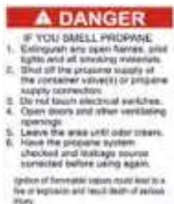
Propane System Label
