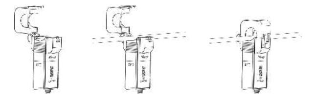
Note: Do not place Phase wire and Neutral wire within a single current transformer.
