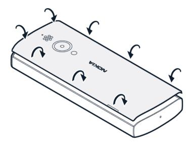
Put back the back cover and press around the edges until the cover snaps into place.
