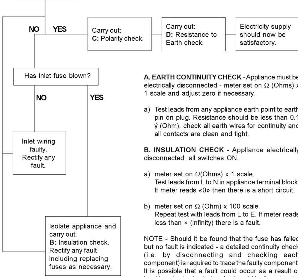
**A. EARTH CONTINUITY CHECK** - Appliance must be electrically disconnected - meter set on  $\Omega$  (Ohms) x 1 scale and adjust zero if necessary.
