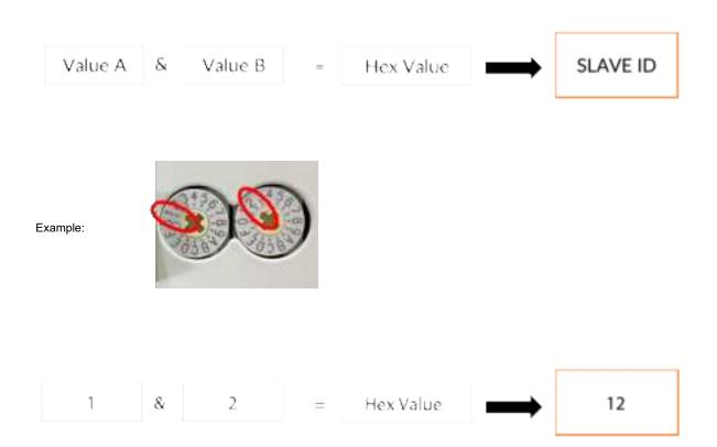
**Important Note:** The combination of 0 and 0 or F and F are not functional. Please ensure these configurations are avoided to maintain proper operations.
